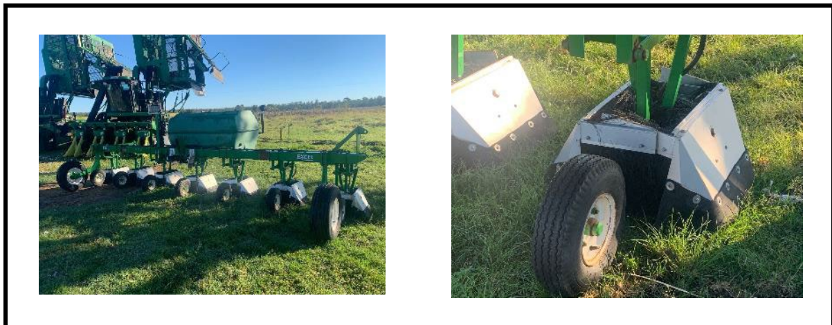
Figure 11: Precision inter-row sprayer with shields in Maryborough.
