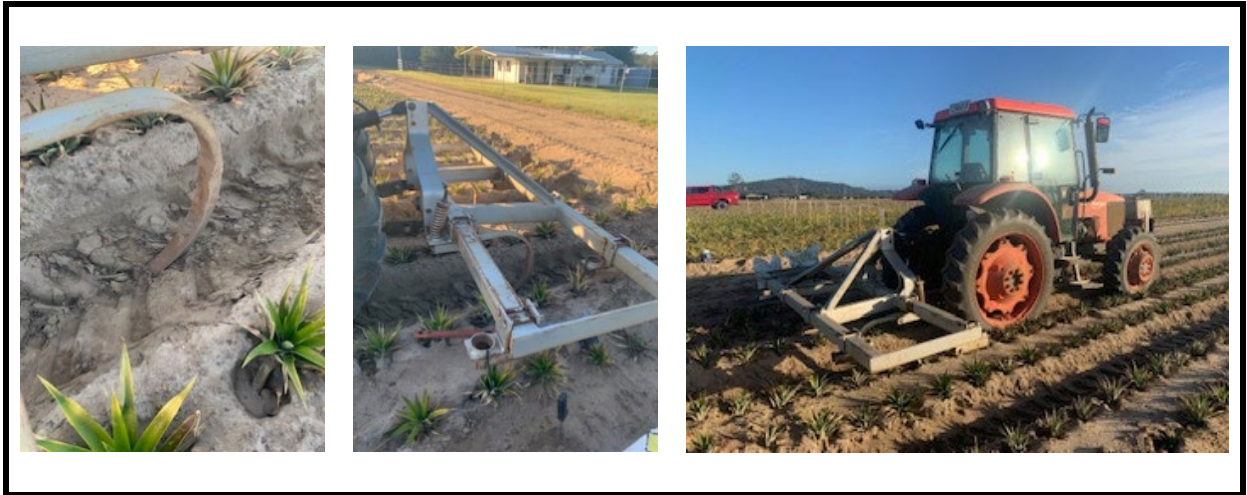
Figure 1: Opening the furrow for before planting seed (left), Implement used to open furrow (middle) and opening the furrow (right).
