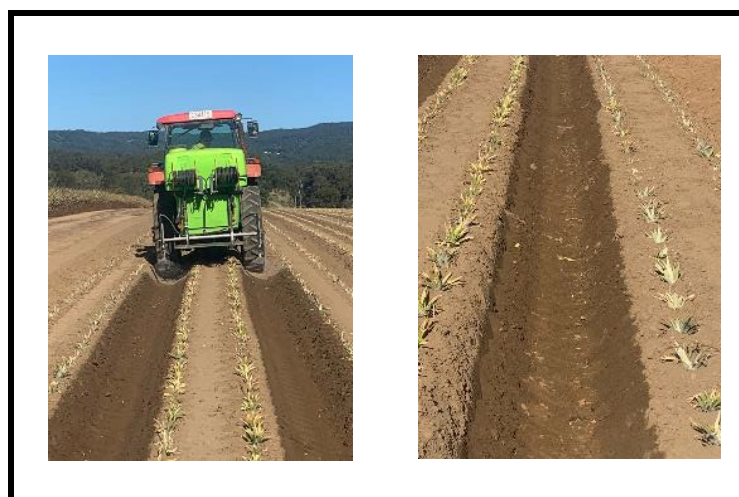
Figure 9: Field testing of upgraded industry headland sprayer showing precision inter-row spray pattern.
