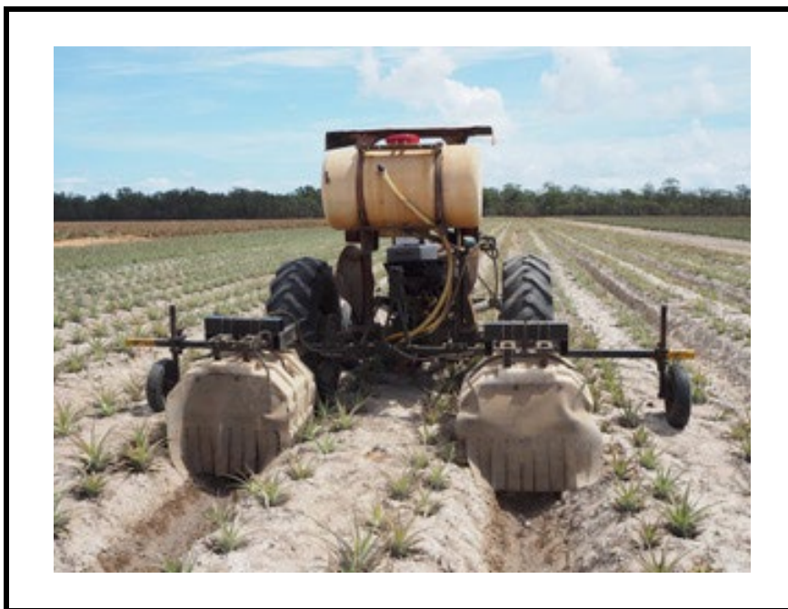
Figure 10: Precision inter-row sprayer with shields in Bundaberg.
