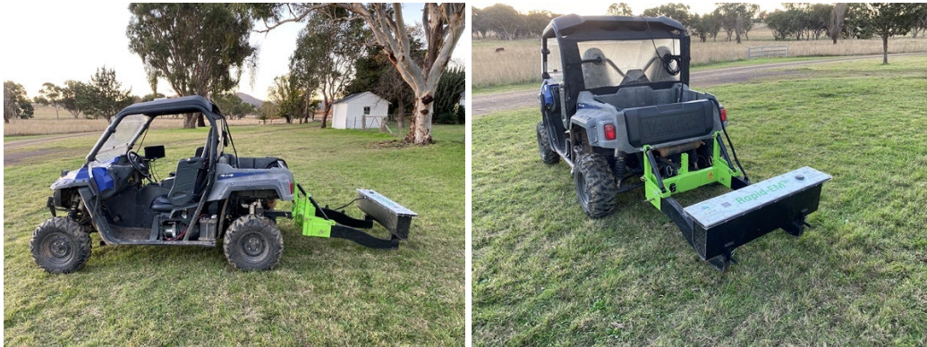
Figure 5: Electromagnetic (EM) unit used to scan the soil (left and right).
