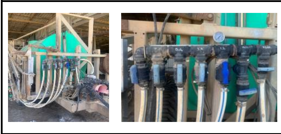
Figures 4-5: (Amaryllis Farming Company) Variable rate and sectional control boom spray set up showing plumbing (left) manual sectional controls (right).
