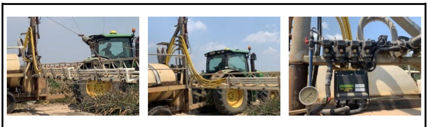
Figures 1-3: (Fullerton Farms) Variable rate and sectional control boomspray (left), boomspray plumbing (middle), automated sectional controls (right).
