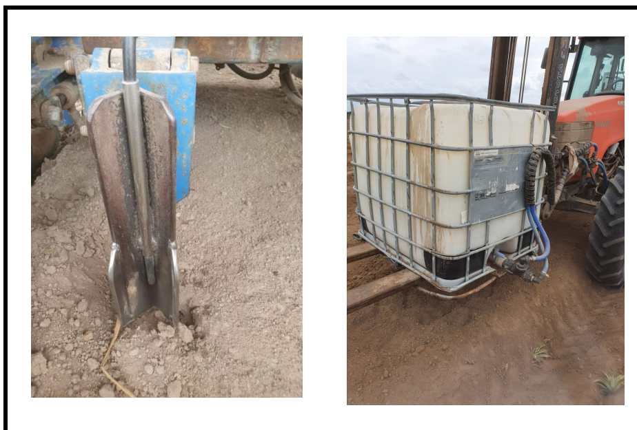
Figure 2: Injector attached to spade on planter (left). Reservoir on front of planter (right).
