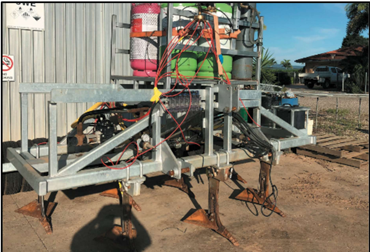
Figure 3 Fumigation rig used to apply treatments.
