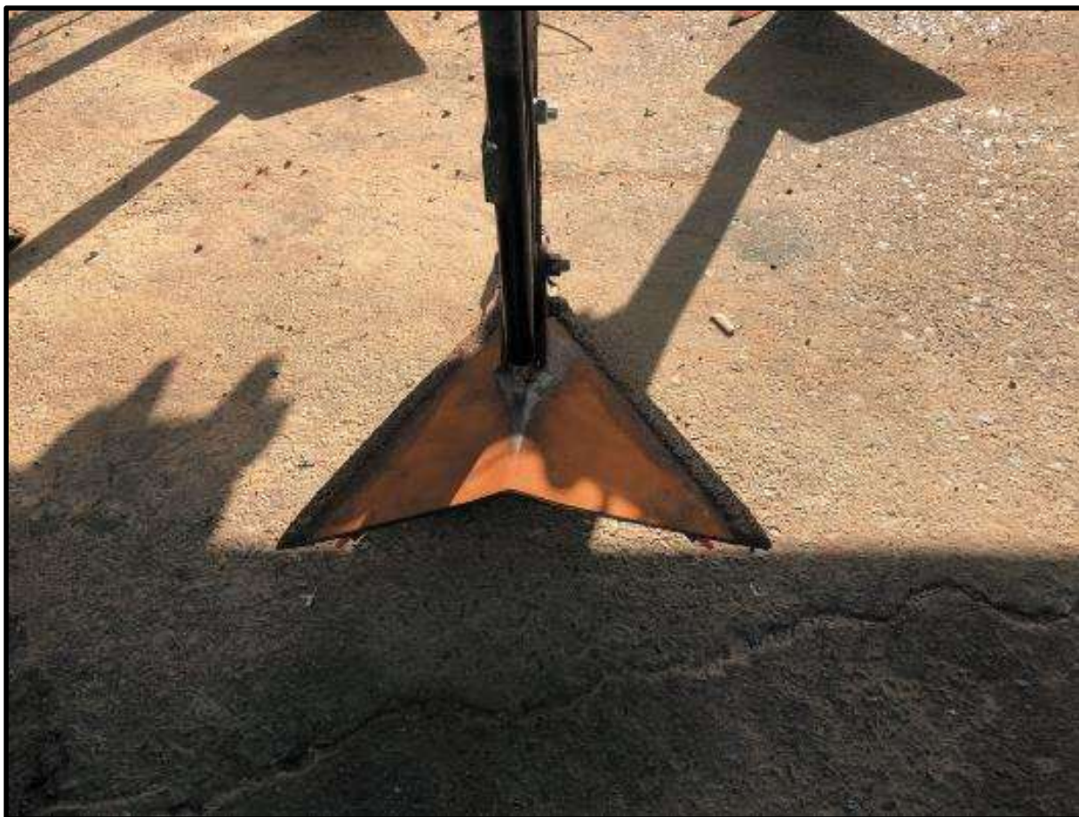
Figure 4. Duck foot tine with dual outlets which can be seen as the two red tubes towards the back of the foot.
