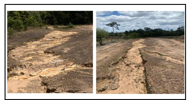
*Figure 8: Treatment 2A - scouring within drain at 12 months (left). Drain one month after installation (right).*
