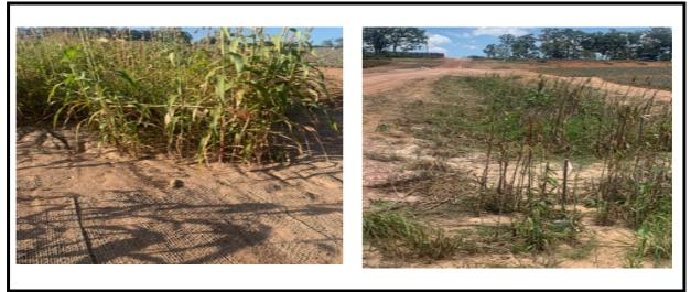
*Figure 10: Treatment 2C - eroded soil captured on jute mesh (left). Vegetated drain at 12 months (right).*
